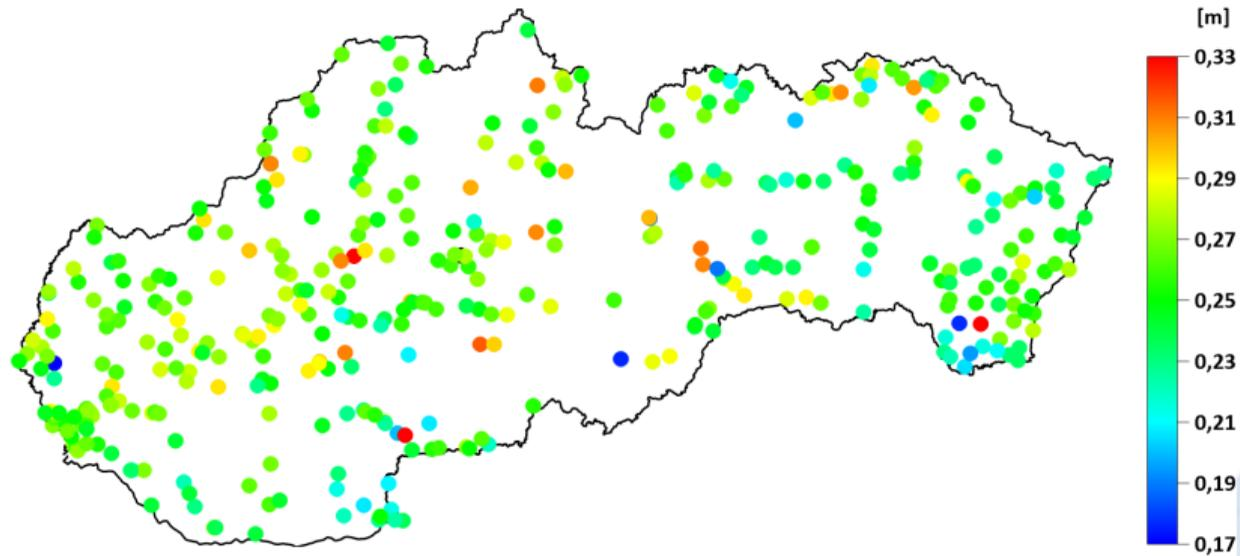
Figure 6: GNSS/levelling benchmarks with differences between the obtained local quasigeoid model and DVRM05.
