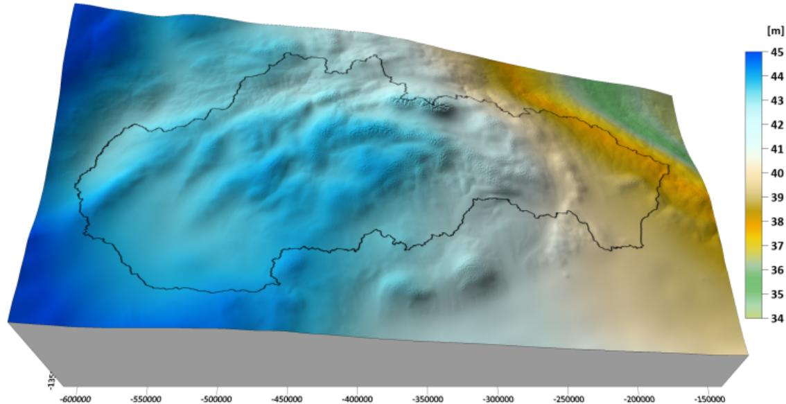
**Figure 5:** Local quasigeoid model in Slovakia as the FEM numerical solution of FGBVP (the horizontal resolution: 100 m x 100 m)
