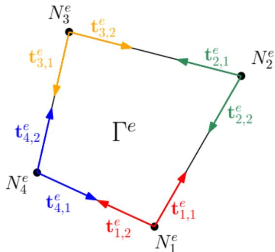
Figure 2: Illustration of tangent vectors  $t_{i,j}^e$  to bottom boundary  $\Gamma^e$  at nodes  $N_i^e$  of an element  $\Omega^e$ .
