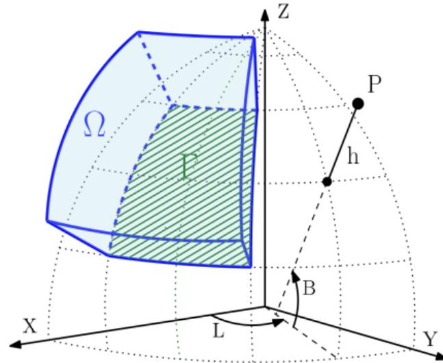
**Figure 1:** The computational domain  $\Omega$ . The domain  $\Omega$  is delimited by blue edges; the bottom surface  $\Gamma \subset \partial\Omega$  hatched by green colour represents a chosen part of the Earth's surface;  $B, L, h$  coordinates denote ellipsoidal latitude, longitude and height, respectively.
