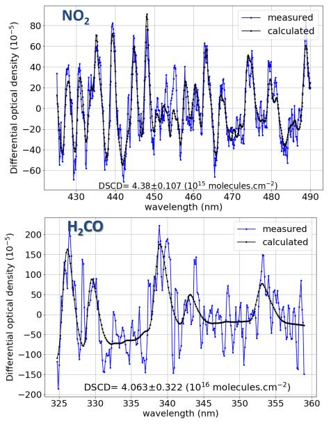
A reference spectrum recorded at 12:17 local time (LT) on 1 June 2020 was used as the Fraunhofer reference spectrum (FRS) for all the retrievals to determine slant column densities (SCDs).
