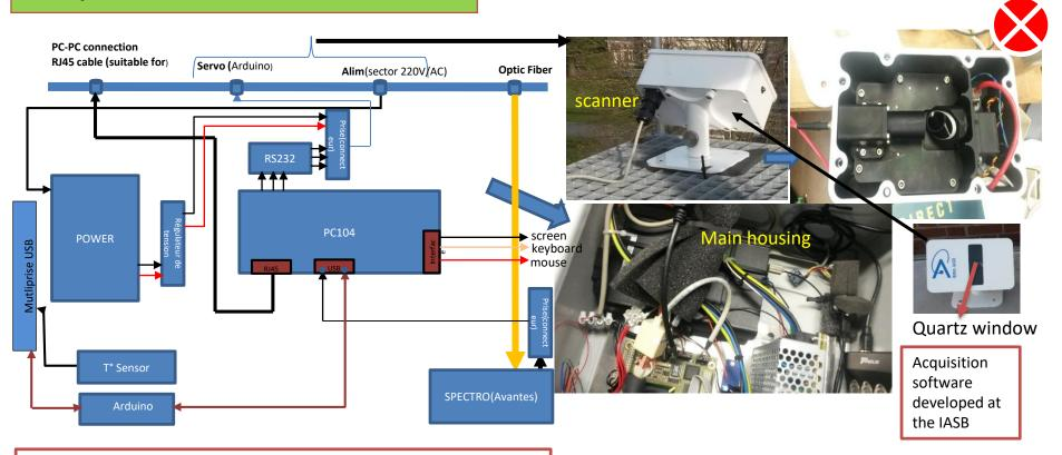
spectro(280-550 nm, 0.7 nm FWHM), PC(104), Power supply with regulation, Acquisition Arduino card, connector (cables et plugs). 600  $\mu$ m diameter fiber optic, 220V/AC, ethernet, RS-232 scanner control over RJ-45.
