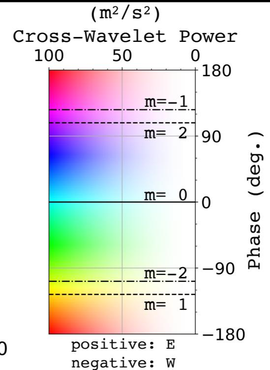
dominant wave number can be resolved through phase-differencing by cross-wavelet analysis between the two stations (He et al., 2018)
