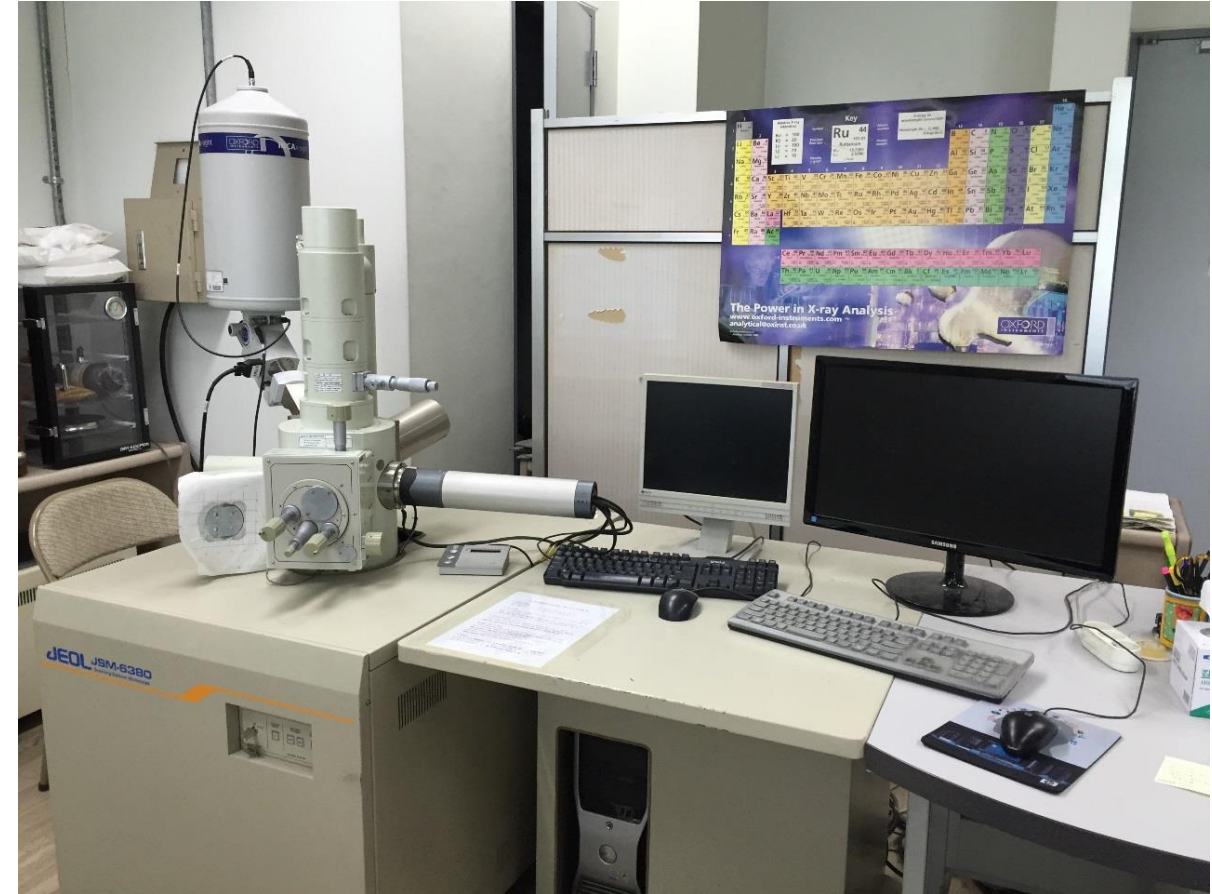
JSM-6380 SEM with HKL EBSD system in SNU
