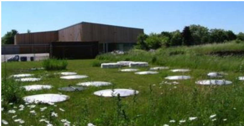
Lysimeter columns: pollutant fate and treatment (diagnostic, risk evaluation, in situ soil treatment, soil restoration)
