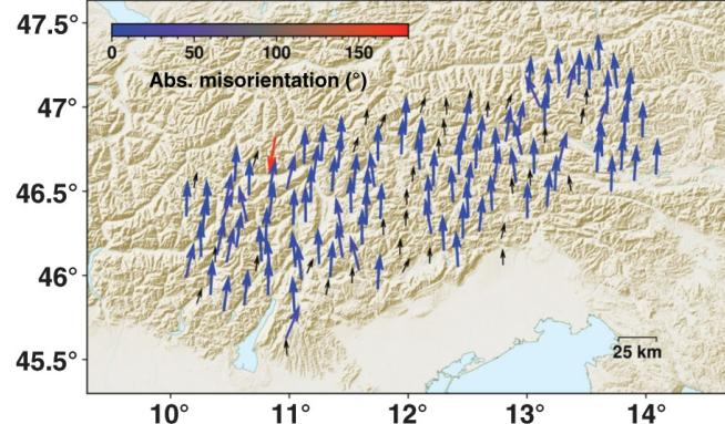
The orientations of the horizontal components of all stations are indicated by the vectors.
