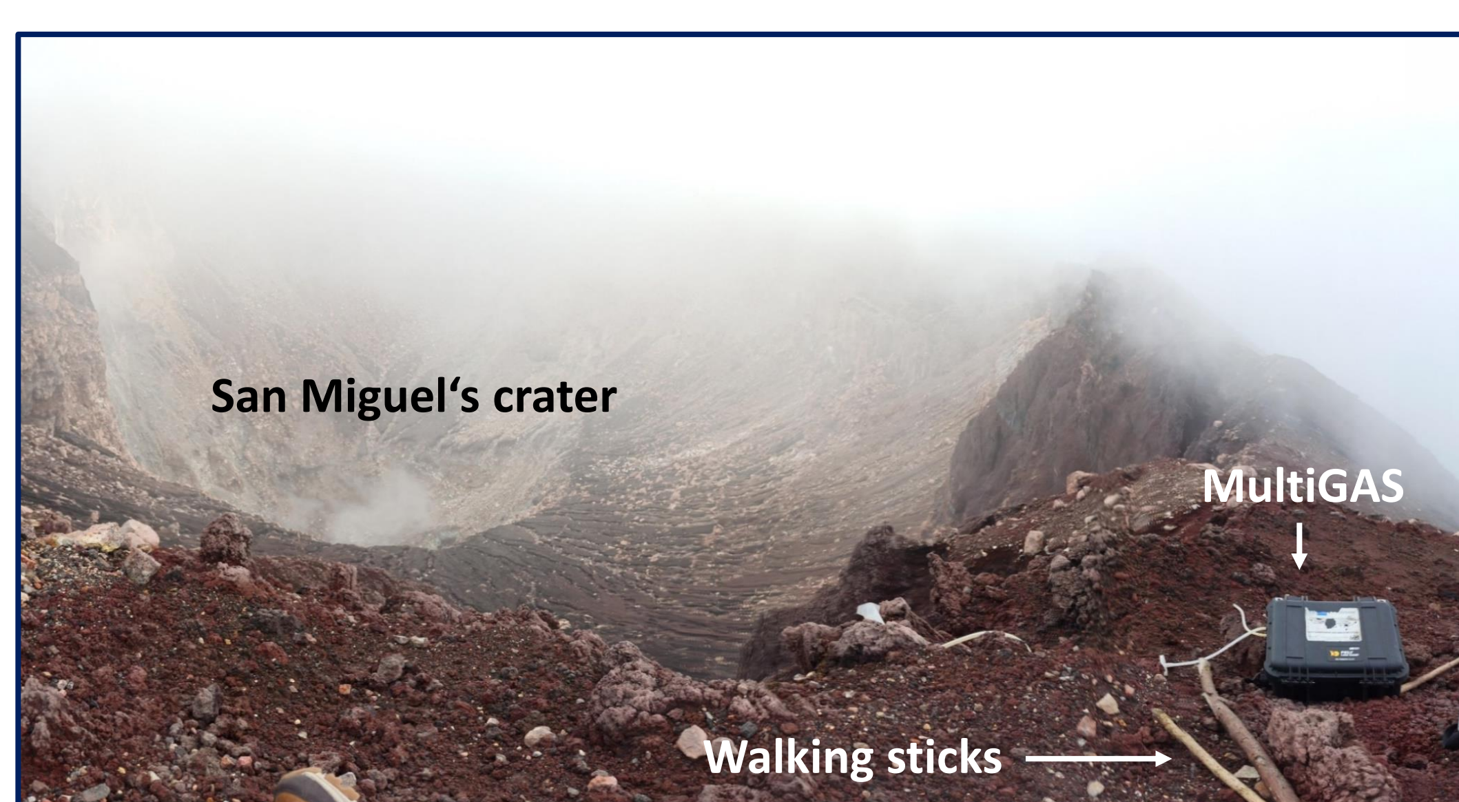
Figure 2. Portable MultiGAS system used for measurements at San Miguel volcano's rim in December 2020.
