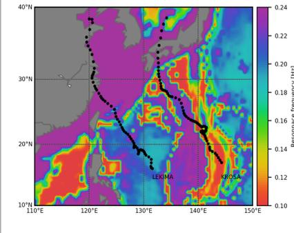
Figure 3 : Source site effect : Map of resonance frequencies within the frequency band (0.10-0.24 Hz) in the region of interest.
