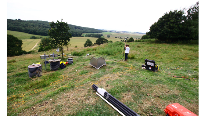
Installation of corner reflectors. (Photo: A. Novellino)
