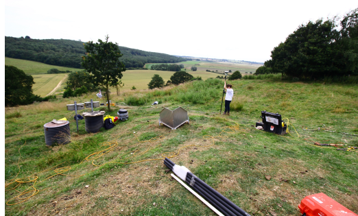
Installation of corner reflectors. (Photo: A. Novellino)
