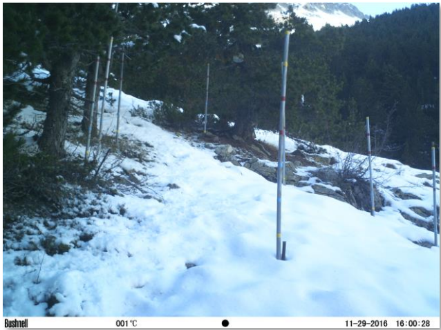
Relative location of the test plots in the valley with semi-automatic snow depth (SD) measurement: Time-lapse camera and snow-poles.
