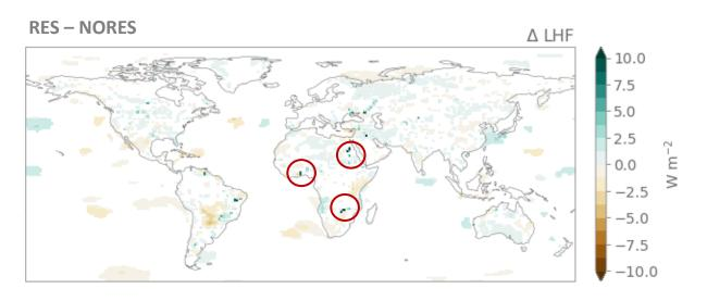
Overall increase in LHF, localized to reservoir grid cells
