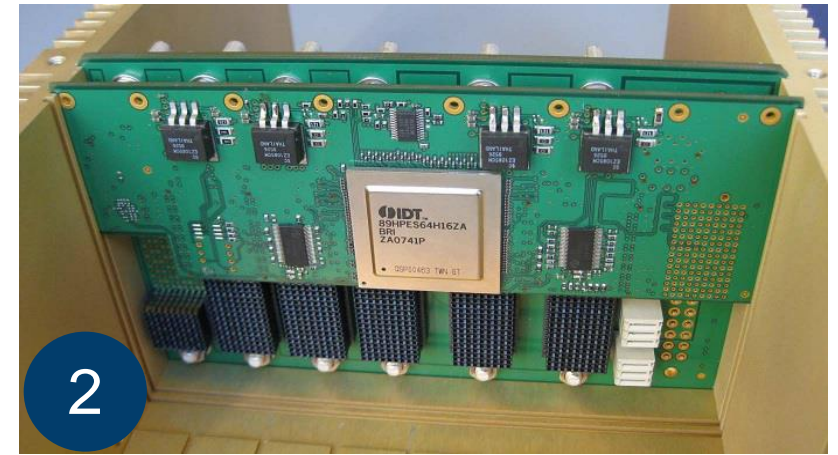
6-slot VPX Backplane with integrated x8 PCIe-switch mezzanine board
