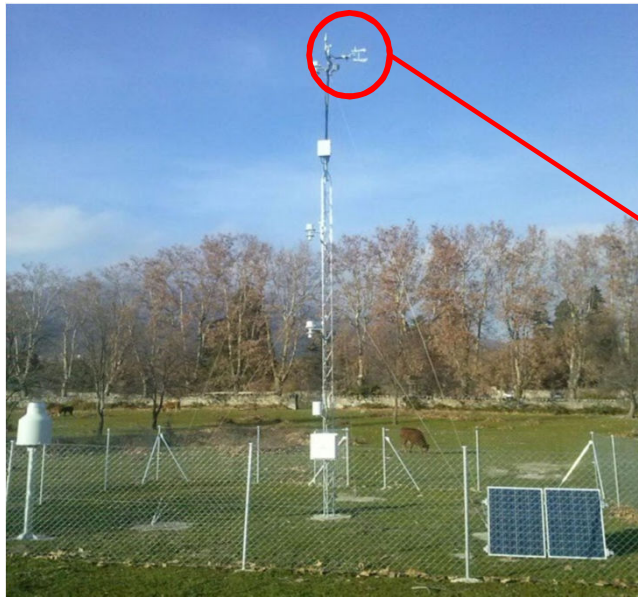
Figure 4. Station scheme (right) and a picture (left) of our at station EG010-La Herrería automatic weather station, located in the municipality of El Escorial at 920m.a.s.l. In the middle, enlargement of the 3D sonic anemometer, Irgason. Atmospheric instrumentation have been design to study boundary layer evolution and CO 2 fluxes.
