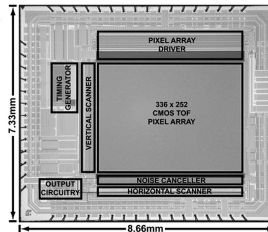
Shoji Kawahito et al. A CMOS Time-of-Flight Range Image Sensor With Gates-on-Field-Oxide Structure
