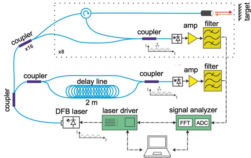
Multichannel lidar diagram
