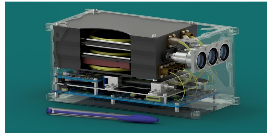
Currently we are working on IVOLGA instrument which is a heritor of MLHS with the purpose of remote sensing of CO<sub>2</sub> concentration and wind speed measurements in Venusian mesosphere in Shukrayaan-1 mission framework
