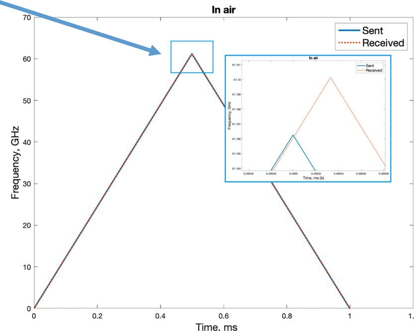
Simulation of sent and received laser signal. Distance to target is 5 m, speed is 3 m/s
