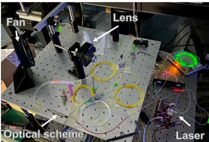
Receiving signal reflected from spinning fan
