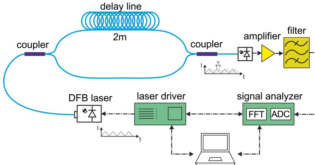
Delay line optical scheme for frequency chirp linearization
