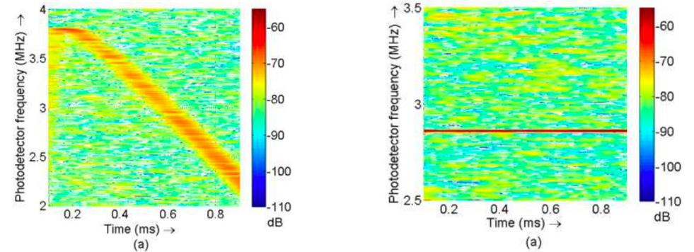
(a) Measured spectrogram of the output of the loop photodetector when the PLL is off; (b) when PLL is on. [Naresh S. et al, Precise control of broadband frequency chirps using optoelectronic feedback]
