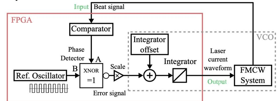
PLL algorithm schematic for FPGA. [Fabian M. M. et al, Frequency-modulated laser ranging sensor with closed-loop control]
