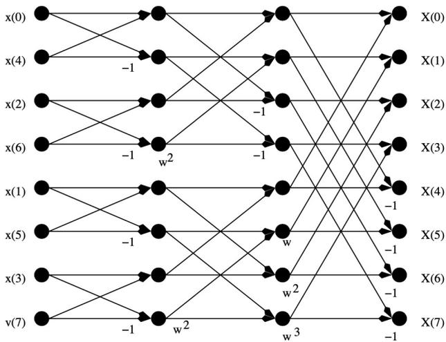
Signal flow through the FFT core
