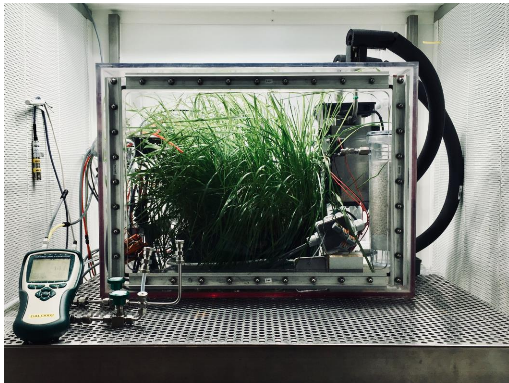
FIG.1 Scheme of the microcosm used for the terrestrial biosphere model (1: Tedlar bags 2 : CO 2 , temperature and pressure sensors 3 : CO 2 injection valve 4 : sample collection valve 5 : Heat exchanger, connected to the temperature sensor 6 : water bath, heated by the heat exchanger 7 : Festuca arundinacea plants 8 : Fan
