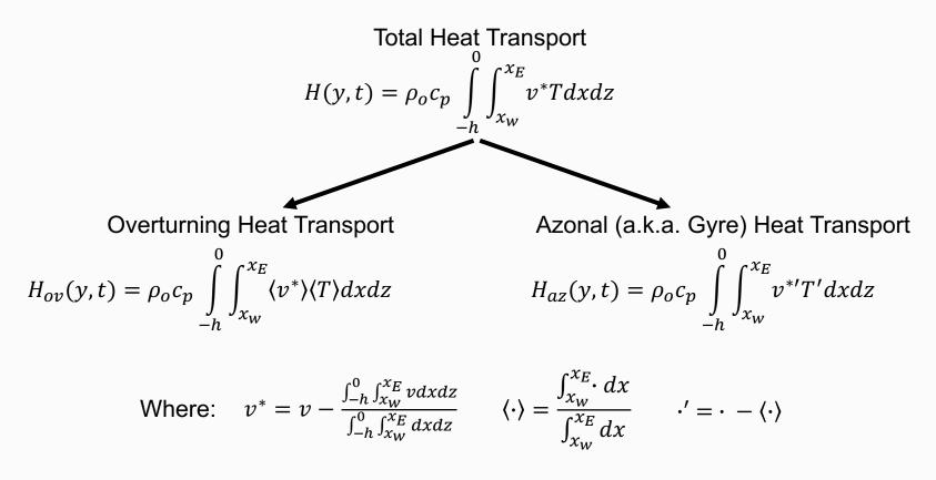
Temperature driven changes: v held constant using 1970-1999 seasonal cycle Velocity driven changes: T held constant using 1970-1999 seasonal cycle Non-linear changes = OHT – Temperature Driven Changes – Velocity Driven Changes
