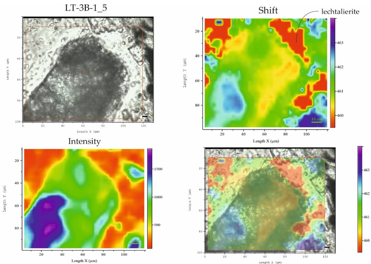
Figure 5: Raman spectroscopy of a quartz grain with a lechatelierite rim showing the internal gradient in the A1 Raman mode shift.
