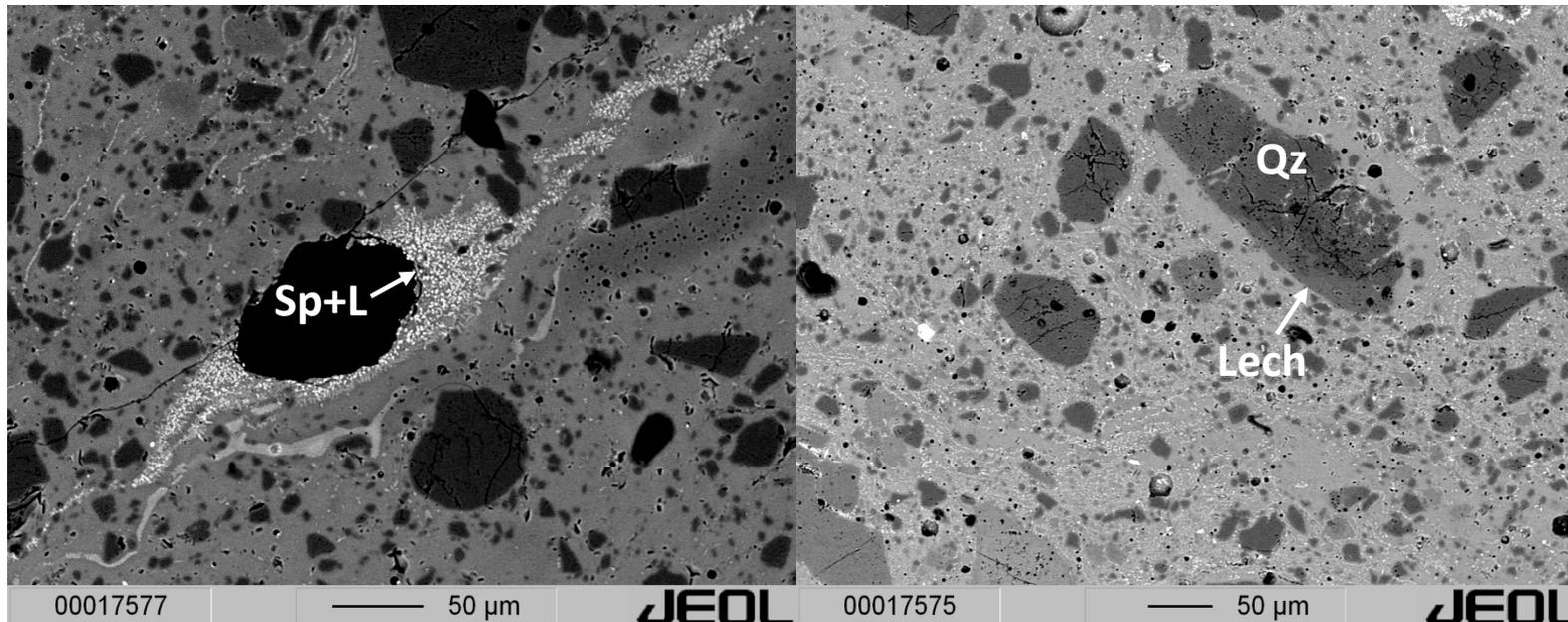
Figure 3: (A) left: biotite breakdown to spinel + glass; (B) right: lechatelierite rim at the edge of a quartz grain.
