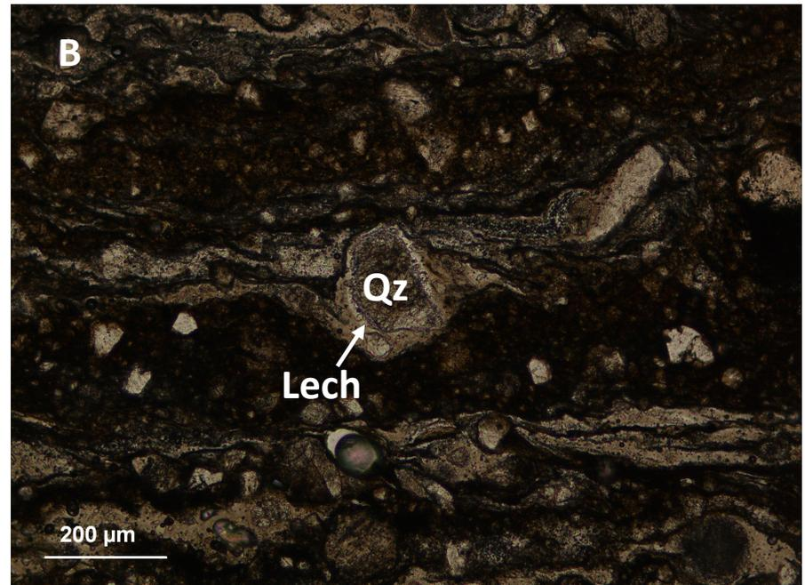
Figure 2: (A) Microphotograph of a frictionite sample (LT-2A); (B) Quartz (Qz) with lechatelierite (Lech) rim.
