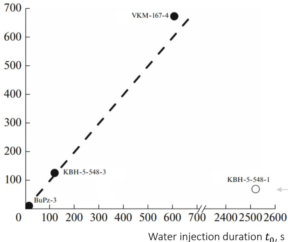
It can be seen that in three of the four samples, the time delay of the AE response approximately coincides with the characteristic time of filling a sample with water. This means that the **time delay of the AE response is mainly determined by the propagation time of the water front.**
