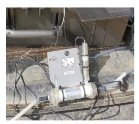
A solubility equilibrium is established between the sampling water and a gas phase separated by this gas-permeable membrane. This membrane is connected to the portable gas spectrometer by one of its capillaries. • • • • • • • • •
