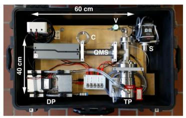
Schematic overview (left) and photo (right) of the miniRuedi mass-spectrometer system (*Brennwald, M et al. (2016)*): 6-port inlet selector valve (S), capillary (C), inlet valve (V), quadrupole mass spectrometer (QMS), turbomolecular pump (TP), and diaphragm pump (DP). The inlet selector valve and the quadrupole mass spectrometer are controlled by a computer. The photo shows the miniRuedi mounted in a wheeled hardshell suitcase for transport and protection.
