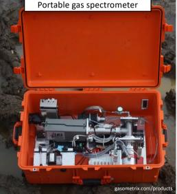
We used a portable gas exchange, membrane-inlet mass spectrometry setup (GEMIMS) which provides countinuous field measurement.
