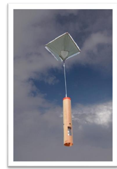
GPS dropwindsondes measures vertical profiles of wind speed, pressure, temperature and humidity during a fall with a frequency of 2 Hz. www.aoml.noaa.gov/hrd/
