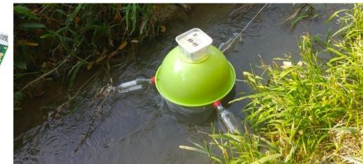
Direct point measurements of  $k$  and  $C_e$ ...
