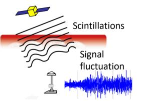
GNSS Signal is disturbed by ionospheric
