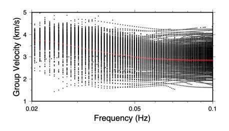
Rayleigh wave group velocity dispersion curves using a random sampling and subset stacking strategy (Schimmel et al., 2017).
