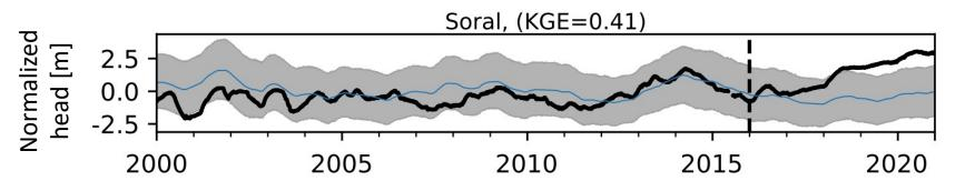
Model structure not suitable to simulate effect of a very thick unsaturated zone (±80 meters)?
