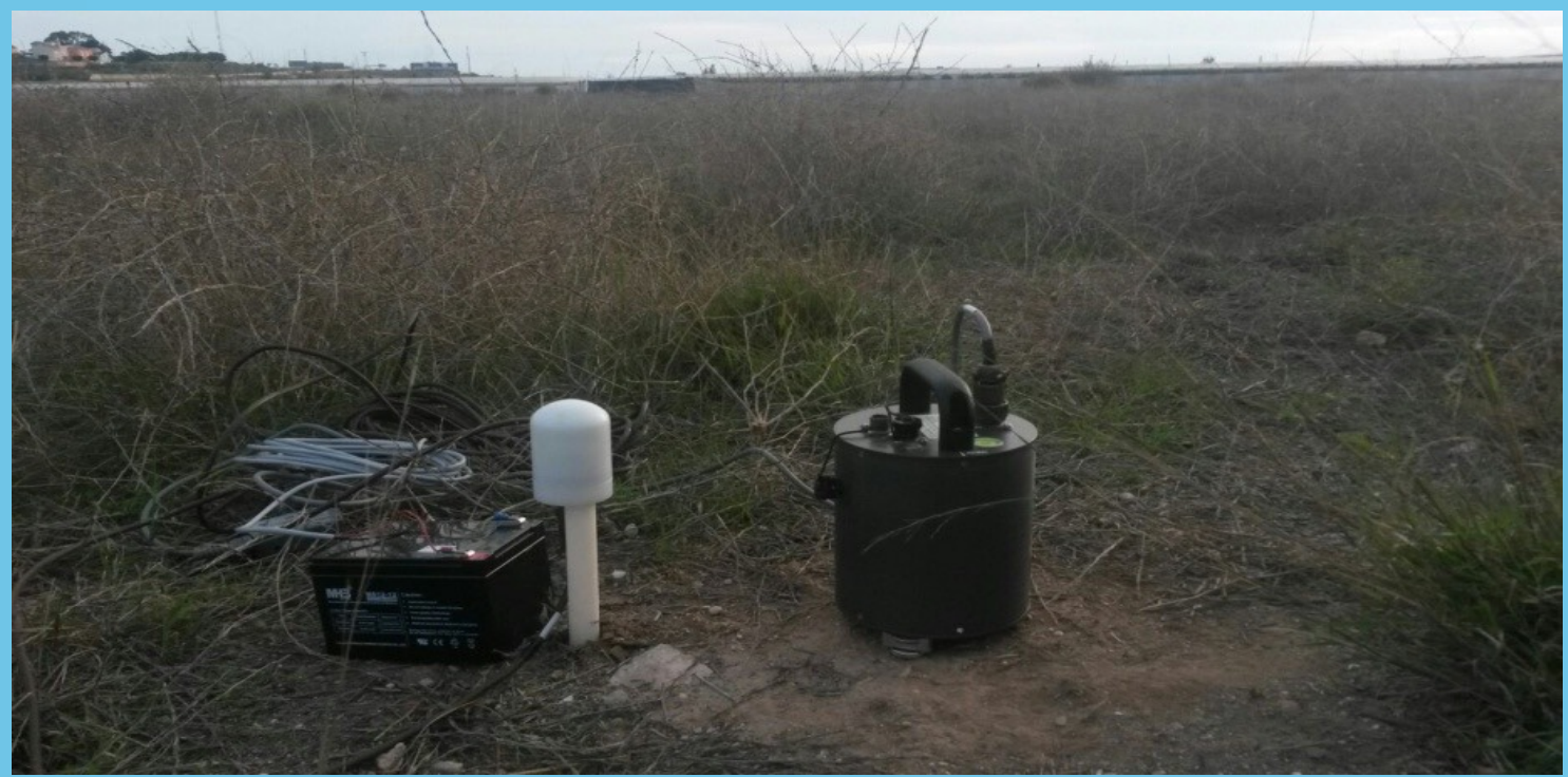
Digital broadband seismometer Guralp CMG-6TD used in long and short time measurements of ambient noise both in El Ejido town and Campo de Dalías basin.
