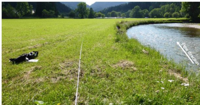
Figure 119: Set up of erosion pin method 2 at the erosion hotspot in the Salza River study area.
