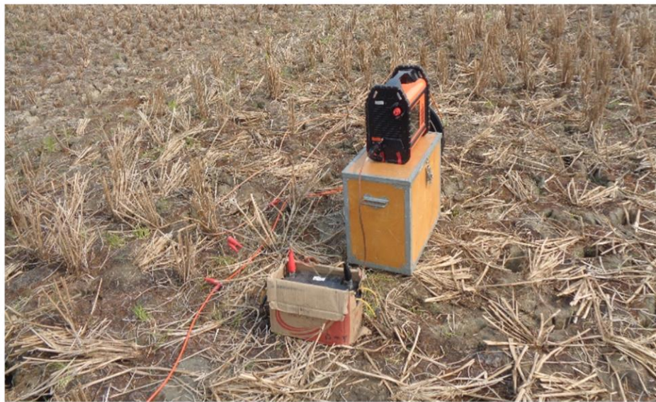
Field Photograph: Resistivity meter setup
