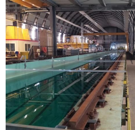
ECN Towing Tank with Resistive Wave Gauges
