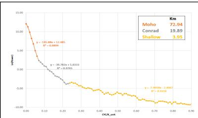
Example of the radial average power spectrum of CBA gravity data for block 1, showing three defined segments (i.e., Moho discontinuity, Conrad discontinuity, and the shallow signal recorded) due to the decay of power with respect to frequency.
