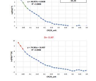
Examples of the power spectrum analysis to estimate the depth to the base of magnetic sources (CPD). Representative 100x100 km2 block (block 34).
