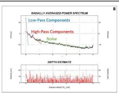
A) The radial averaged power spectrum of the CBA data used to create residual and regional gravity anomaly maps.; B) The radial averaged power spectrum of the RTP data used to create residual and regional magnetic anomaly maps.
