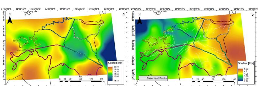
Map results of the layer discontinuities obtained after the power spectra analyses of the Bouguer WGM-12 model. A) 150x150km block grids over the CBA WGM-12 that were analyzed individually to obtain the depth results of the Moho and Conrad discontinuities and the depths of the shallowest records of the signal.; B) Moho discontinuity depth map.; C) Conrad discontinuity depth map.; D) shallowest depths of the recorded spectrum map.
