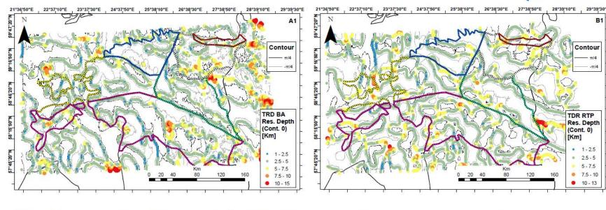
Theoretical depth maps from residual potential data. A1) TDR depth map from gravity data.; A2) SPI depth map from gravity data.; B1) TDR depth map from magnetic data.; B2) SPI depth map from magnetic data.
