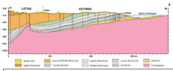
Geology schemes of Estonia. A) Generalized map with the sedimentary cover of Estonia shows outcrop areas of lower and middle Paleozoic rocks. Dash lines correspond to the profiles used to analyze potential data; B) Geological crosssection profile of Estonia. Vertical lines correspond to drill cores.
