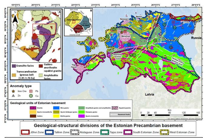
Geological map scheme of the Precambrian basement of Estonia, showing geochemical anomalies according to Soesoo et al., (2020) . A) Major Palaeoproterozoic tectonic domains in the Baltic Sea area (modified after Bogdanova et al., (2015)); B) Crustal segments of the East European craton (modified after Gorbatschev and Bogdanova (1993)).
