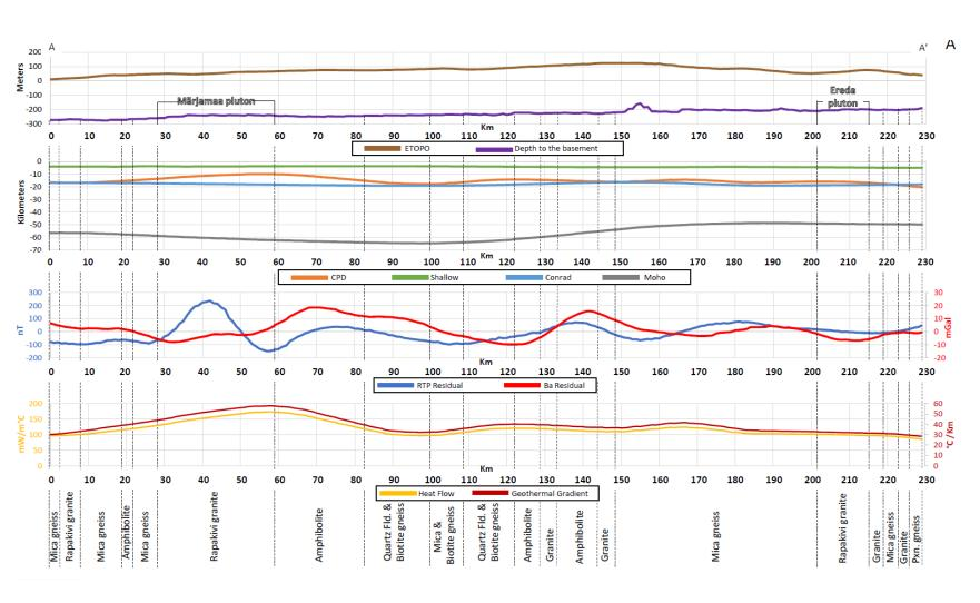
Example of one of the Profiles done across Estonia showing the relations of the topography, crustal layers, residual potential anomalies and heat flow across the basement lithology.
