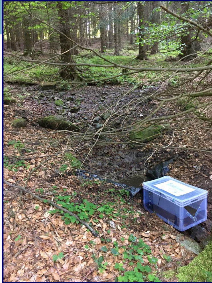
Fig.6: Instrumentation of spring site with a weir for discharge measurements
