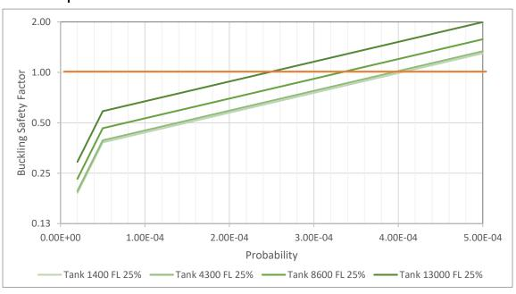
**Tank buckling Factor** = Pr/ Pw ≤ 1
