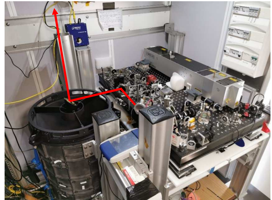
DIAL system integrated in lidar truck
