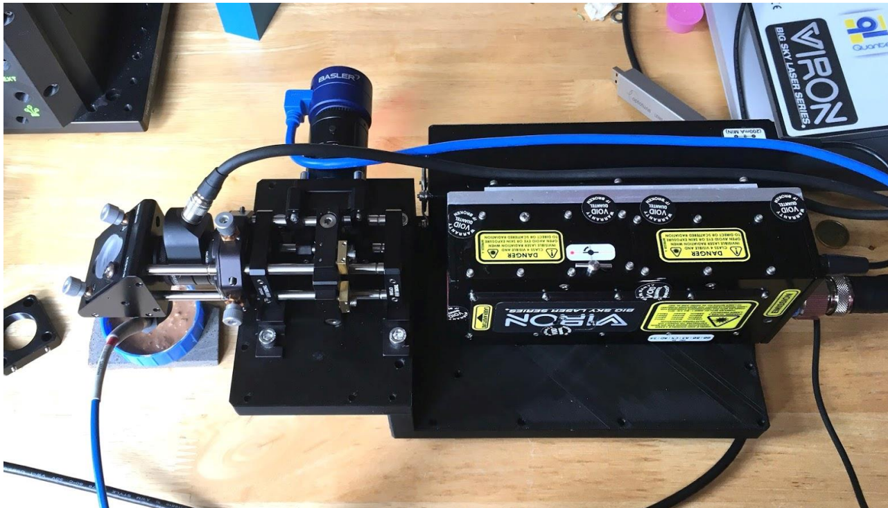
Slurry LIBS spectrometer scale model
