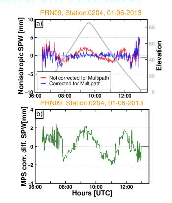
Non-isotropic (left) slant precipitable water vapour with multipath correction (in blue colour) and without multipath correction (in red colour) and their differences shown in dark-green colour for station 0204
