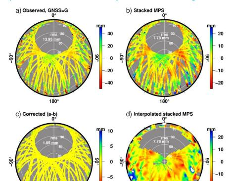
The multipath stacking supresses elevation and azimuth dependent site-specific multipath effects.
