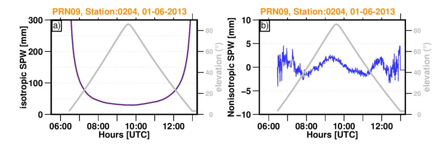
The isotropic (left) and non-isotropic (right) slant precipitable water vapour. The non-isotropic contribution can reach 10% of the isotropic component.
