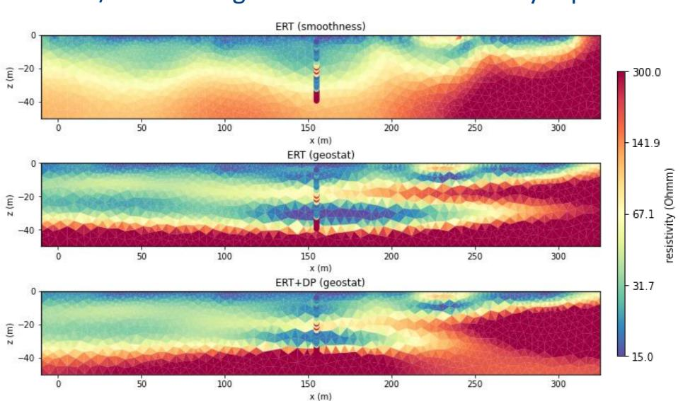
Inversion result with classical smoothness, geostatistical regularization (Ix/Iz=50/5m) and with DP data.
