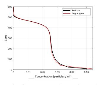
Implementation in the LES model as an external module in parallel to Eulirian approach
