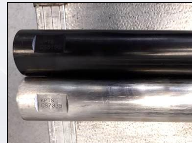
Logging tool came black out of the well
