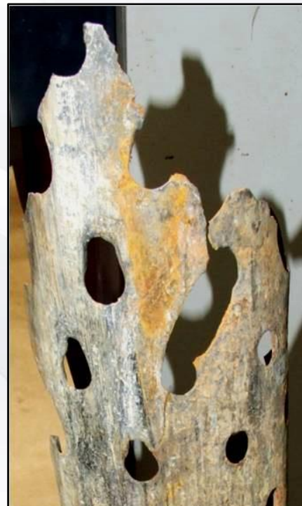
Corroded liner due to mixing of fluids from two feed zones
