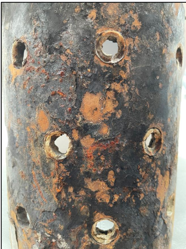
Clogged holes in liner from well in N-Iceland
