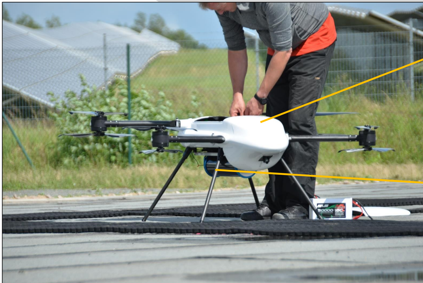
Fig. 03: Drone-Detector-System on a calibration pad of Wismut GmbH in Thuringia, Germany.
