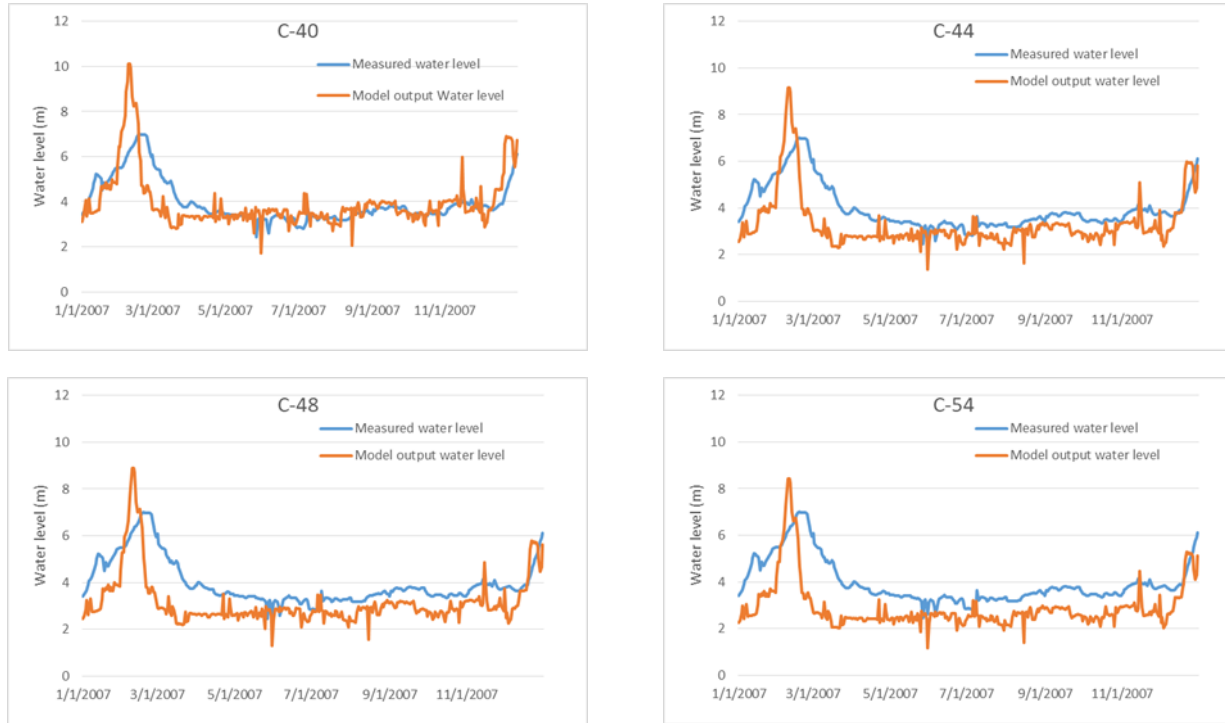
Figure 9: Measured and simulated water level at Marromeu in 2007 including morphological simulation and dredging for a different Chézy's value
