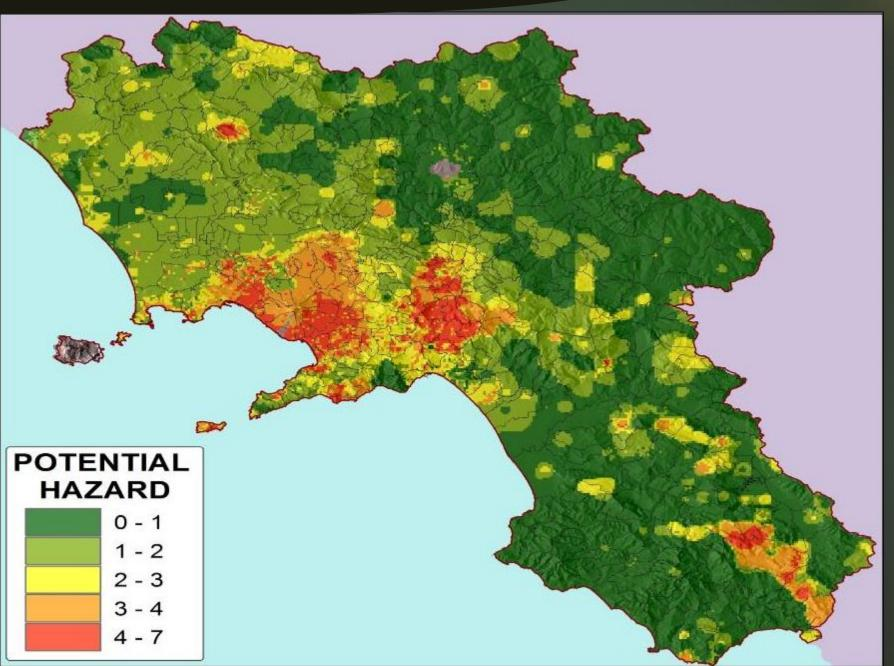
The Potential Hazard (PH) map was generated for potentially toxic metals using the criterion of exceeding (H = 1) or non-exceeding for the residential use of soils (Legislative Decree 152/2006), pixel x pixel.
