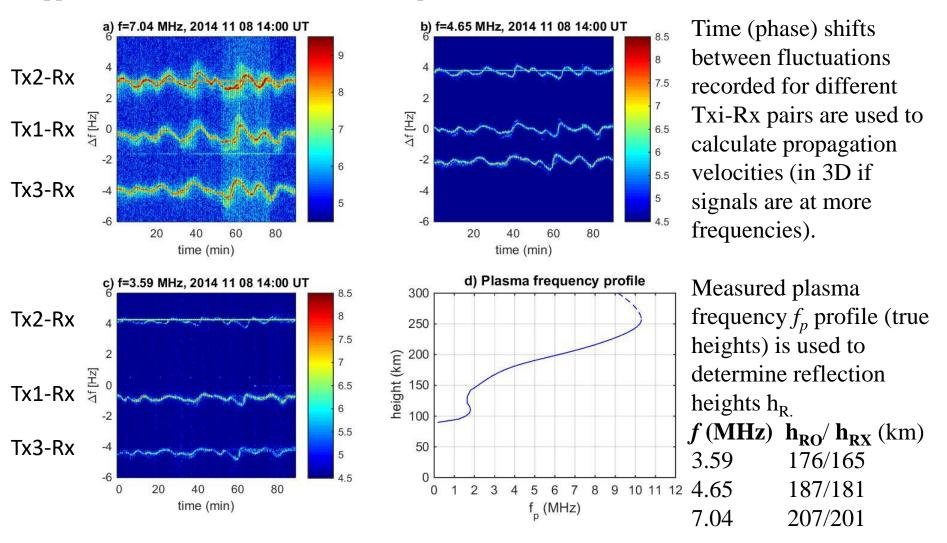
First, maxima of spectral intensities for each transmitter are evaluated to obtain Doppler shifts as single-valued functions of time.
