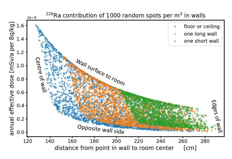
Wall thickness = 0.2 m Density = 2350 kg/m3
