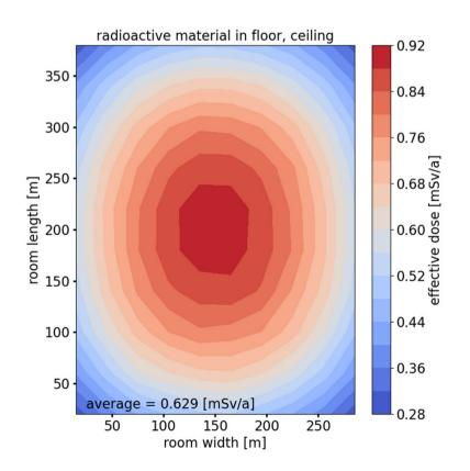
Wall thickness = 0.2 m Density = 2350 kg/m3
