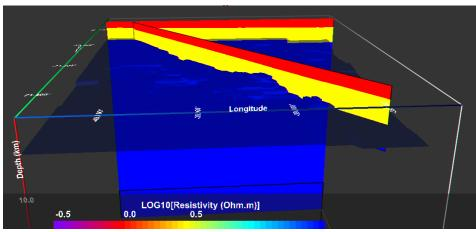
**Scenario II)** incorporating the Salt layer and the reservoirs thicknesses and resistivities
