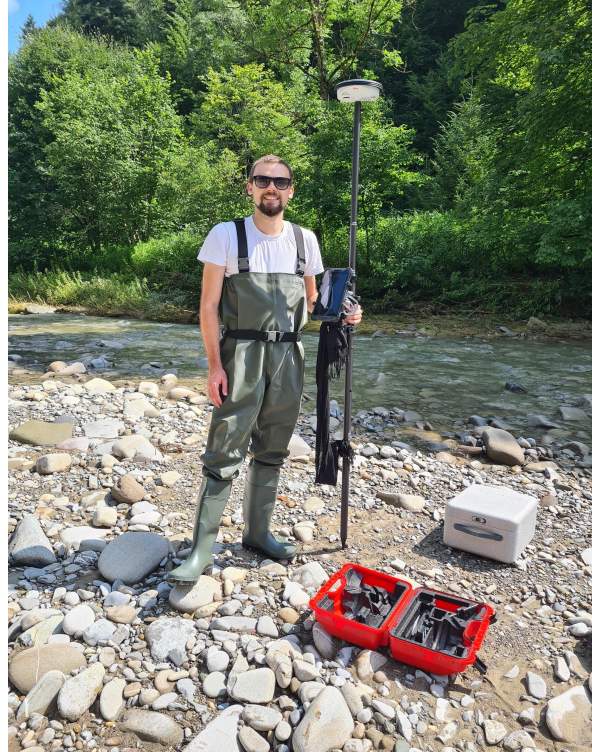
GNSS Leica Zeno GG04 Plus Accuracy of c. 2cm
