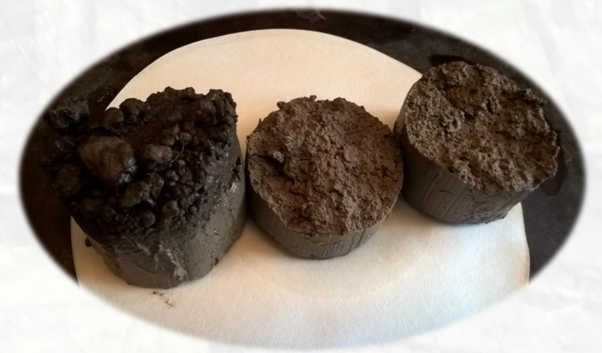
Soil columns design in the laboratory filtration experiment: aggregates were not water resistant; an in-growth mesh bag increased the filtration capacity of the column.
