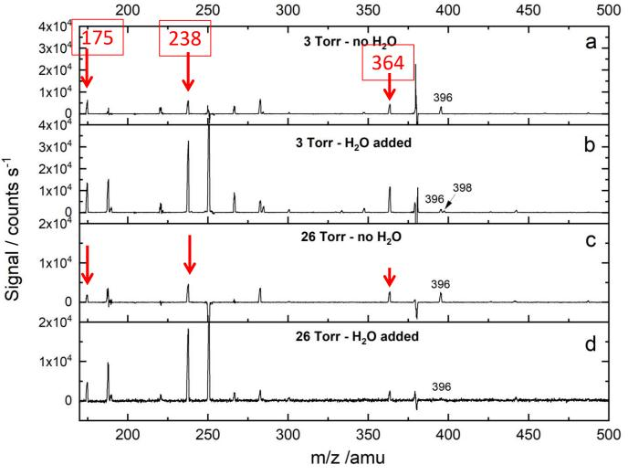
The nitrate reagent ion signals increase with water: a correction of product signals is needed.
