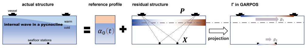
$$\Gamma(t, \mathbf{P}, \mathbf{X}) \equiv \alpha_0(t) + \alpha_1(t) \cdot \frac{\mathbf{P}}{L^*} + \alpha_2(t) \cdot \frac{\mathbf{X}}{L^*} \qquad \begin{cases} g_1 = \alpha_1 V_0 \\ g_2 = \alpha_2 V_0 \end{cases}$$
