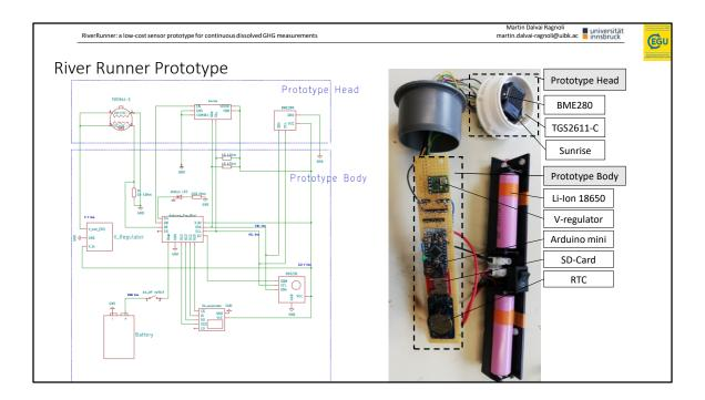
The Prototype consist of two parts: a sensor head and a sensor body. The latter houses all the electronics and the battery.
