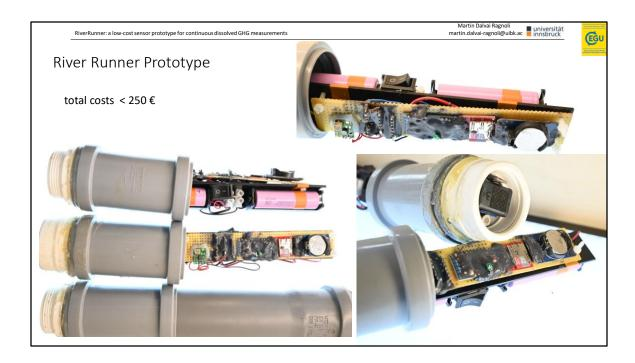
The Prototype Body is completely waterproof inside PP based tubing.
