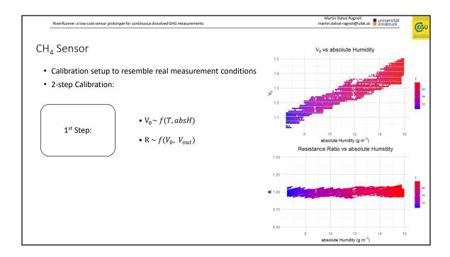
First step: Sensor reference output voltage (V0) at background atmospheric CH4 levels is modelled. V0 is dependent from T and humidity
