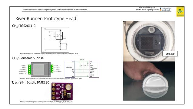
The prototype Head houses the gas sensors:
