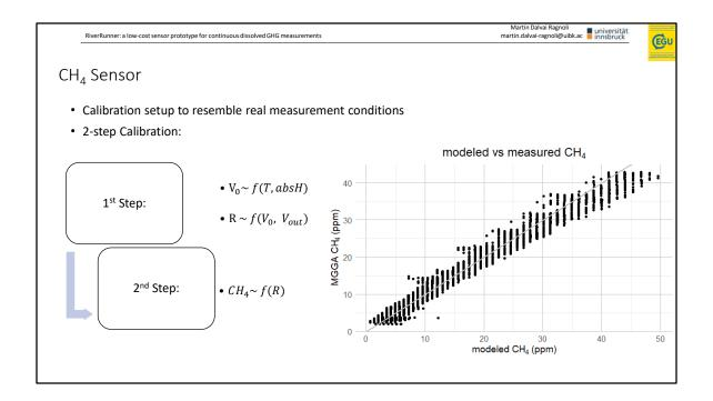
Second step: stepwise introduction of methane. Mole fraction of CH4 is modelled based on R
