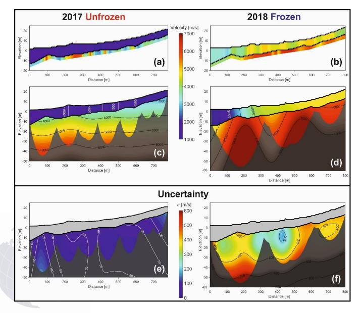
Two independent surveys (a, b) shows the same lithological boundary using short offset refractions with different geometries
