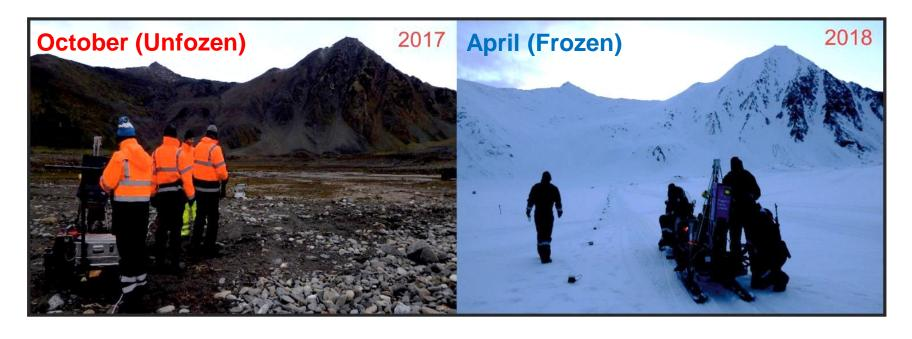
Two Arctic expeditions were organized to perform time-lapse seismic. For both seasons equipment (seismic source, deployment of stations) had to be prepared in different way. Special sledges were constructed for snow use.
