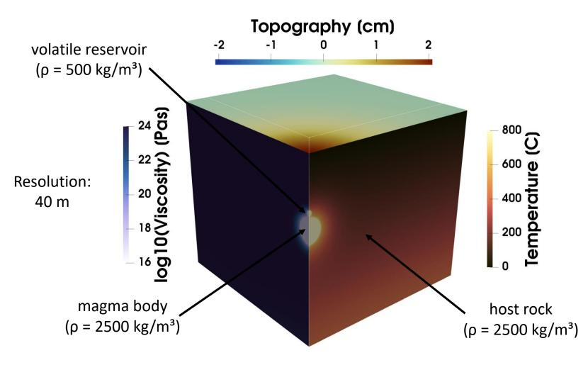
Eruption is approximated by instantly replacing buoyant volatiles with non-buoyant magma
